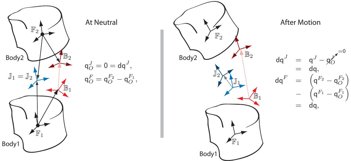
In the figure, the body centers of geometry are situated at the body origins frames ( $\mathbb{F}_1$  and  $\mathbb{F}_2$ ), and the joint orientation and `orientation_in_parent` both equal zero. This allows us to use the relative motion between the joint frames ( $\mathbb{J}_1$  and  $\mathbb{J}_2$ ) to specify the change in relative motion between the centers of geometry.
