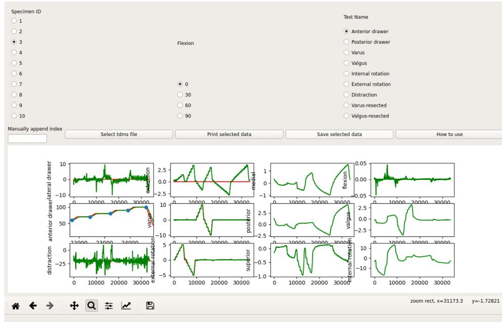
Fig. 3.1: The GUI of the the semi-automatic process of extracting experimental data.
